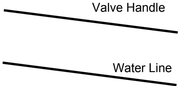
Our valves are CLOSED (preventing water to flow through the valve) when the valve is TURNED (or perpendicular) to the water lines.
