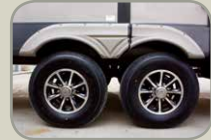
Contemporary aluminum rims with E-rated radial tires.
