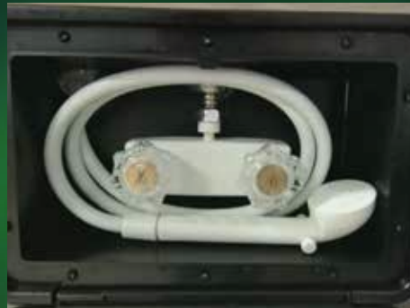
Outside Shower With Hot And Cold Water
