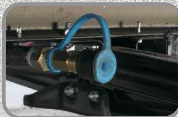
Outdoor Grill Quick Disconnect
