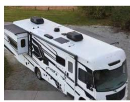
**FIBERGLASS ROOF** One-piece seamless fiberglass roof with extended rain spouts; more durable and easier to maintain than TPO or rubber.
