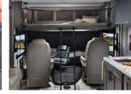
HIDE-AWAY POWER OVERHEAD BUNK Power foldaway overhead bunk with ladder and safety net. 350 lb. weight limit with an abundance of storage.
