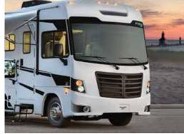
AUTOMOTIVE BONDED WINDSHIELD/SMALLEST A PILLARS IN CLASS Our windshields (with lighted logo) are automotive bonded and wrapped in steel to allow for 6" A pillars for better visibility.
