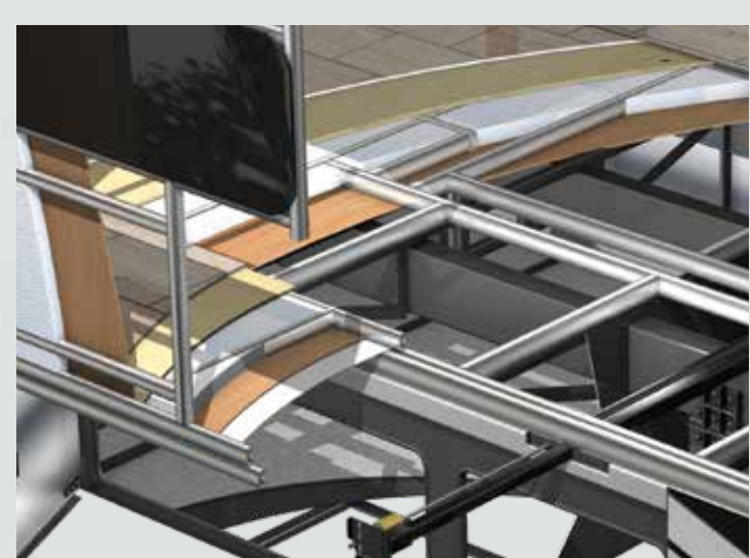
3 1/8" THICK FLOOR INCREASES RIDE QUALITY, REDUCE ROAD NOISE, ADDED RIGIDITY TO THE FOUNDATION
