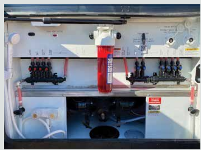
WATER MANIFOLD SYSTEM OFFERING POINT TO POINT CONNECTIONS, EQUALIZED WATER PRESSURE & TEMPERATURE, AND THE ABILITY TO ISOLATE ANY ISSUE
