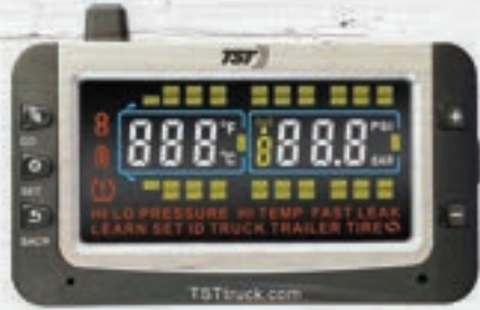
TST TIRE PRESSURE MONITOR SYSTEM Standard on all Cedar Creek Fifth Wheels is the TST tire pressure monitoring system that alerts you to any tire problems while on the road.
