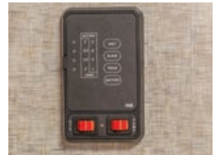
Monitor Panel for Tanks and Battery Levels
