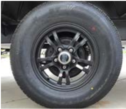
14" Tires for improved towing in place of 13"
