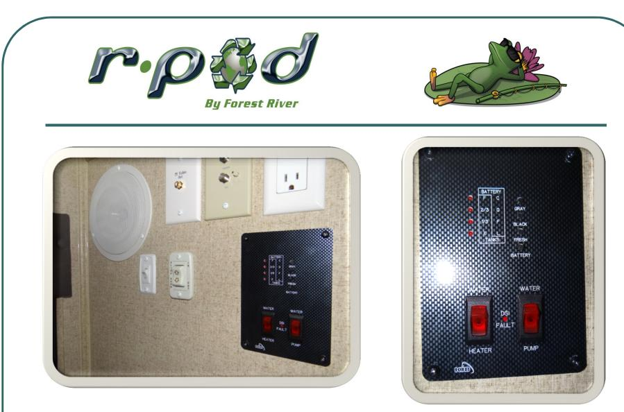
This is the r-Pods control center. Here you control interior ceiling lights, the electrical slide out mechanism, hot water heater, water pump and battery/holding tanks levels. This is a simple and easy way to control several features of a r-Pod.
