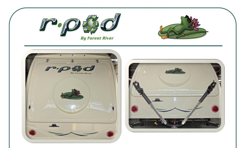
These are photos of the rear garage r-Pod models (RP-181 and RP-182). All r-Pod's have a rear spoiler with LED lights. The photo on the right portrays the optional bike rack. This rack holds two bicycles and mounts to the rear hitch of the r-Pod. (2 bikes only)
