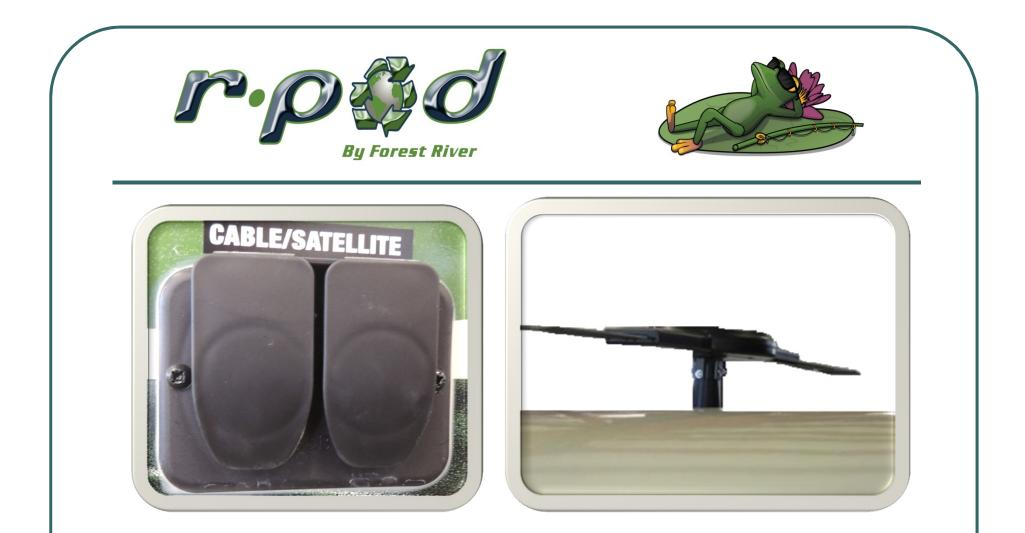
r-Pods are pre-wired for cable and satellite television. r-Pods are also equipped with a high-definition digital multidirectional antenna. The antenna is also <u>not</u> a crank-up antenna. Enjoy watching the best quality television available at your campsite in your r-Pod.
