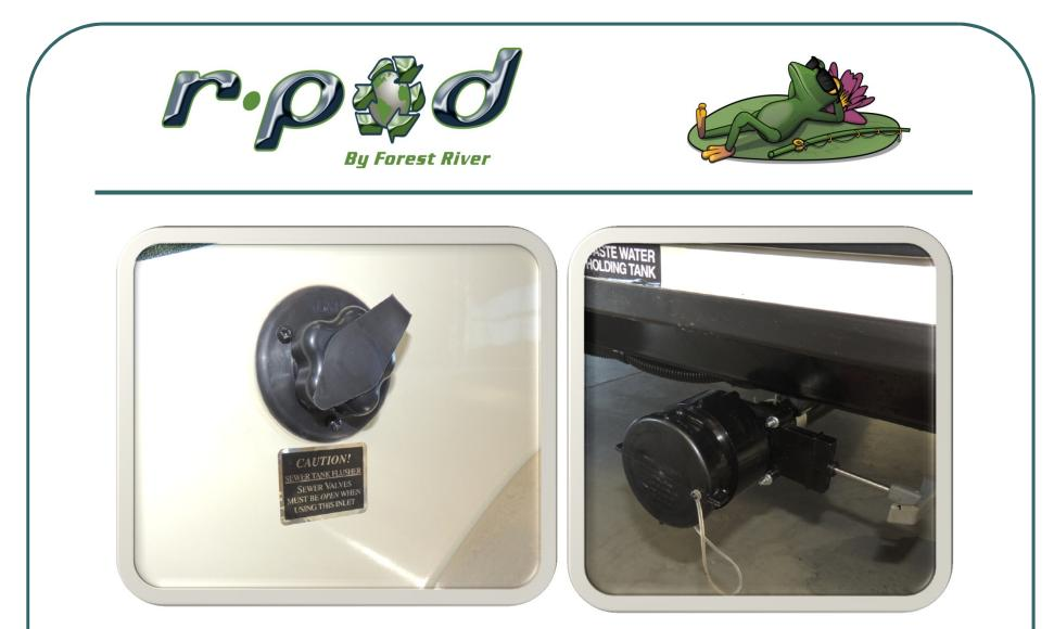
Here are two features found on all r.pods. On the left is the black tank flush hook up and on the right is the black tank dump valve. To use your black tank flush, simply hook a garden hose to the black tank flush receiver and turn your hose on. Sewer hoses easily attach and detach from the dump valve (seen on right), making it a less messy task.
