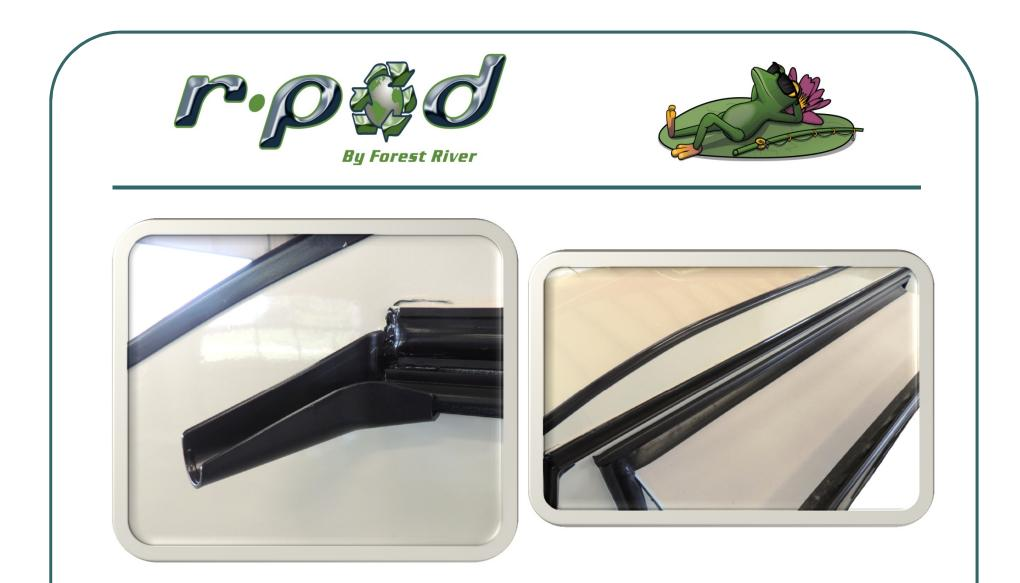
Above r-pod slide outs, there are extended drip rails. These act as gutters to keep rain water from running off the roof onto the slideout.
