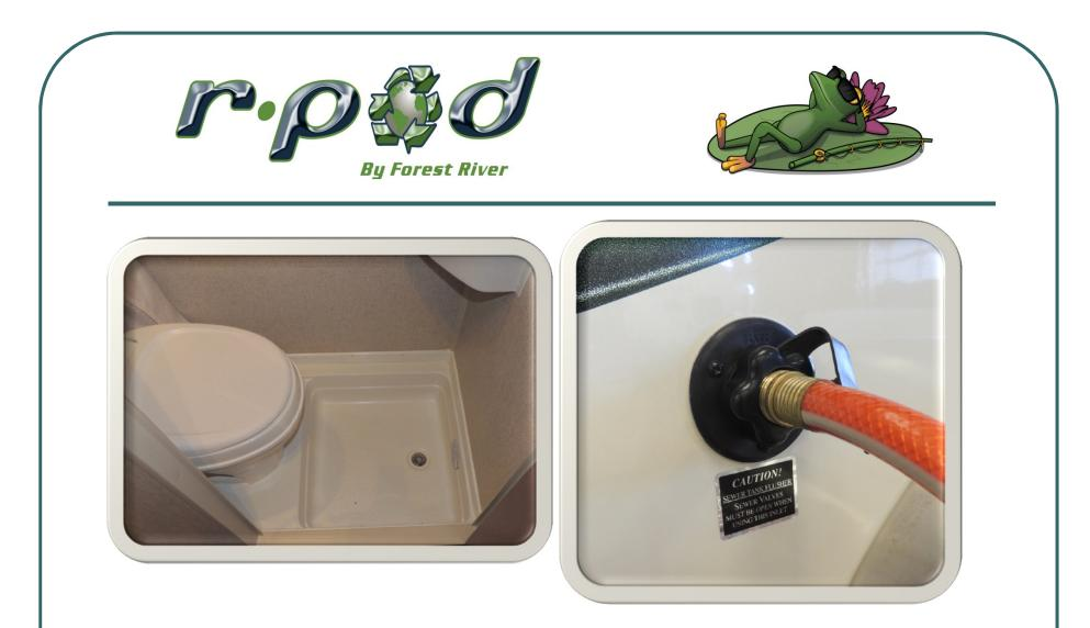
r-Pods wet bath provides you your own facilities, functional and private. All r-Pods are equipped with a standard black tank flush system. This is a "must-have" to maintain the integrity of your black tank and to prevent human waste from solidifying and blocking your dump valves.
