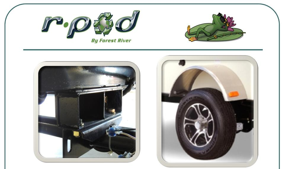
r-Pods offer an optional axle riser. This option will lift your r-Pod 3 ½" additional inches above the torsion axle suspension. R-Pods have 14" aluminum wheels with radial tires and electric Nev-R-Adjust brakes.
