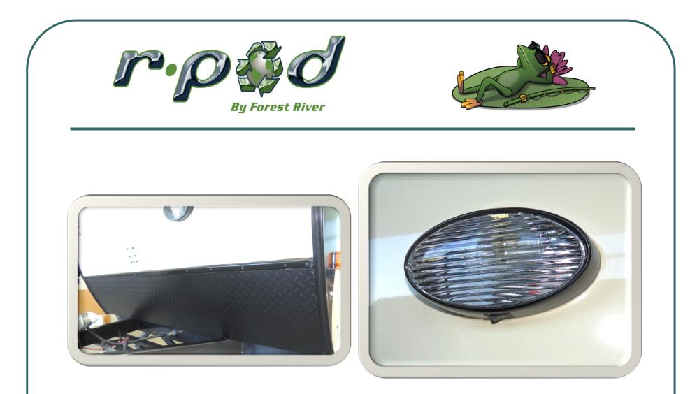
All r-Pods are equipped with a black diamond-plate shield on the front end. These offer great protection from rocks, pebbles and other road debris from damaging your front end. Also included is a front docking light so you can illuminate your r-Pod's A-frame in the evening.
