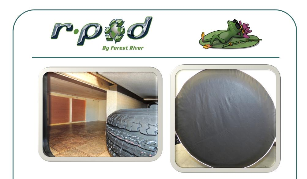
All r-Pods have standard spare tires. Spare tires are full-size and are mounted on the rear (right) of the r-Pod or inside the pass thru storage (left).
