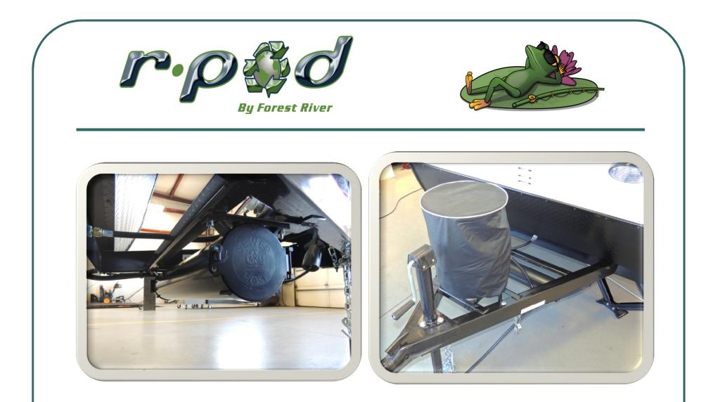
These are photographs of the r-Pods A-frame on the front of the RV. The A-frame has an easy to use manual tongue jack. On top, there is a 20# LP tank and a dual battery rack. Underneath, there is a sewer hose storage compartment.
