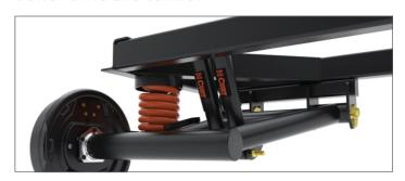
Gas shocks dampen spring oscillations for improved ride quality and vehicle handling
