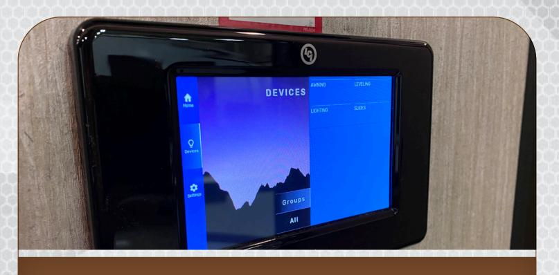
CENTRALIZED ONE CONTROL SYSTEM FOR AWNING, SLIDES & LIGHTS WITH BLUETOOTH COMPATIBILITY
