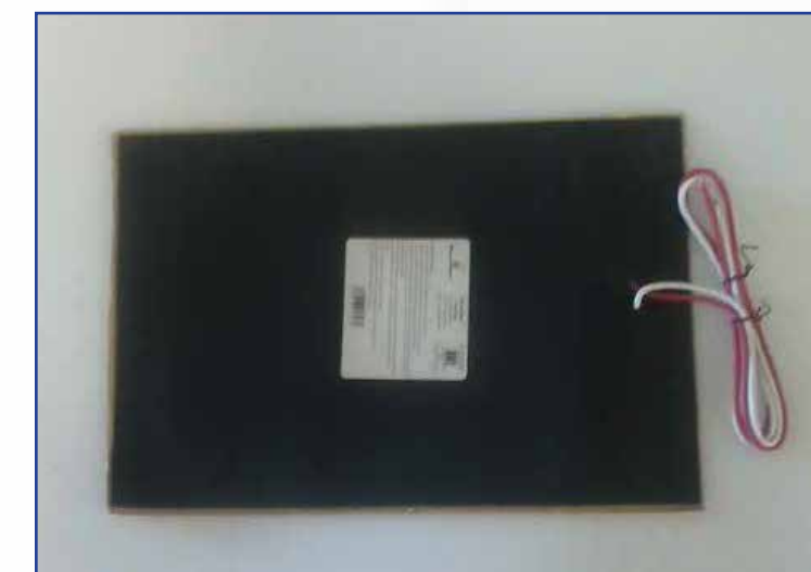
12V Heat Pads on Tanks
