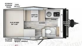
LENGTH: 20' 4" CLOSED HEIGHT: 5' 8" BOX SIZE: 14' HITCH: 353 AXLE: 2309
