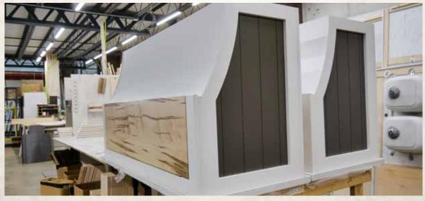
Kitchen cabinets can be one of the most striking features in a new fifth wheel. All of our cabinets are built from quality materials and are hand assembled by in-house skilled craftsmen and women. All lumber core stiles are predrilled and countersunk. This creates long lasting quality cabinetry that will stand the test of time.
