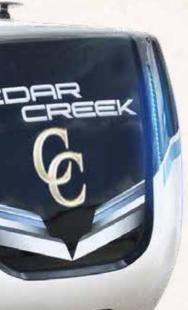
**"TRUE " GELCOAT EXTERIOR** WITH PAINTED FRONT **FIBERGLASS CAP**
