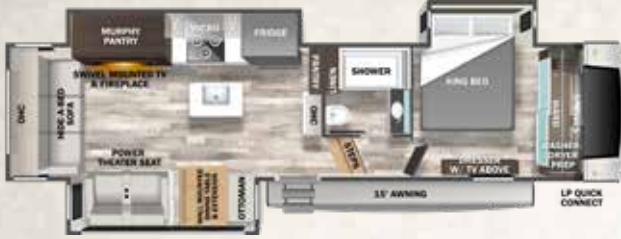
2925RL HITCH WEIGHT-2,343 lb. / GVWR-14,343 lb. / UVW-10,172 lb. CCC-4,171 lb. / LENGTH-34' 11" / HEIGHT-13' 6" / WIDTH-96"
