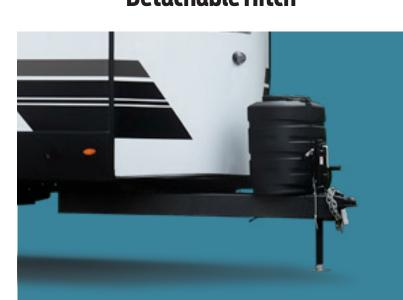
Our trailers come with a detachable hitch, for meeting lot requirements. Quickly unbolt or re-bolt the hitch as needed. (NA 40DUPLEX)
