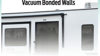
All welded aluminum-framed, vacuum bonded laminated superstructure with 2" insulated walls. Vacuum bonding ensures the complete glue coverage and curing on walls.
