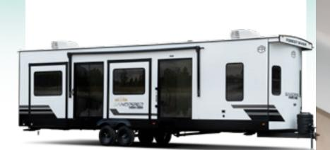
2" thick vacuum bonded walls, foam block insulation, enclosed underbelly, 12 volt heated holding tank pads, and radiant foil help keep our units protected from the seasons.
