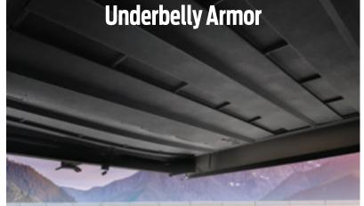
Corrugated panels offer extreme protection from road debris, water and other hazards. The panels can be disassembled quickly for routine maintenance or repairs. Combined with heated holding tanks your tanks will stay warm and clean.
