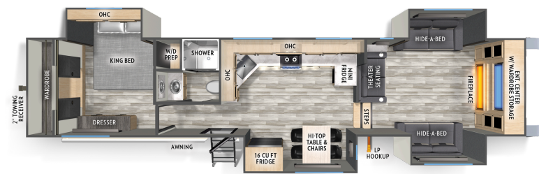
35FL HITCH: 2,115 GWR: 14,115 UWW: 10,708 CCC: 3,407 LENGTH: 43'5" HEIGHT: 13'2" WIDTH: 96" TANKS (F/B/G): 60 38 76 AWNING: 15'
