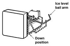
When the ice maker thermostat senses the preset temperature for the ejection of the ice cubes, the fingers will start to rotate, dumping any ice cubes and filling the mold with water. When the storage container is full, the bail arm will come in contact with the ice cubes. The bail arm cannot return to the full down position and the ice production is stopped until the bin is emptied, or ice cubes are removed.
