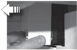
2. Locate the adjusting screw under the protective cover. Turn the screw counterclockwise to increase the size of cubes.
