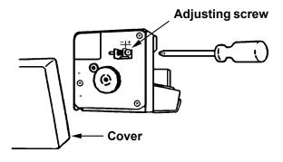
3. Turn the screw clockwise to decrease the cube size or if the mold is overfilling, and the cubes are stuck together.
