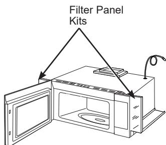
When replacing a 36" range hood, filler panel kits fill in the additional width to provide a custom built-in appearance.
