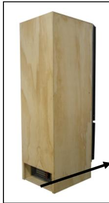
The ventilation on this unit is blown out the front grill by fans installed in the unit. The most efficient ventilation design is for the back to be open to allow cooler air to be drawn over the condensers and out through the front.
