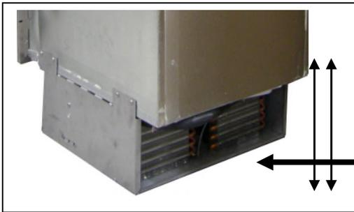
Use a soft brush to clean condenser, using an up and down action gently removing surface dirt.
