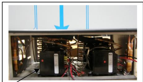
To remove module loosen philips head screw located on the left side of the module, and pull module straight out.
