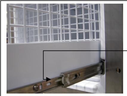
To remove drawer push on the plastic releases on the outside of both the left and right drawer glide and gently pull the drawer towards you.
