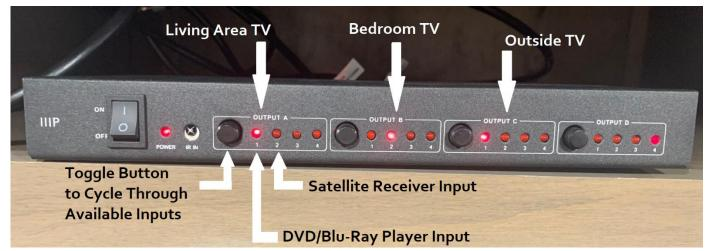
\*In this example – The Living Room TV (Output A) is connected to the DVD Player (Input #1); the Bedroom TV (Output B) is connected to the Satellite Receiver (Input #2); and, the Outside TV (Output C) is connected to the DVD Player (Input #1).
