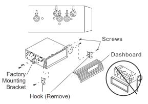
screws at 2 places on each side. Do not exceed M5 x 9 MM maximum screw size. Longer screws may damage components inside the chassis.
