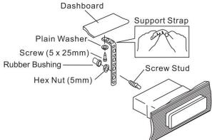
position it. Some vehicle installations provide cavity for rear support. In these applications, place the rubber bushing over the screw stud and insert the radio.
