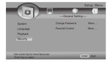
Press the" HOME "button to activate the Setup Menu on screen display Video Monitor Only menu.
