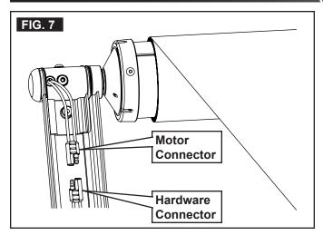
4. Connect 16 Gauge (minimum) wire leads (user supplied) to motor connector, and tape in place (with electrical tape).
