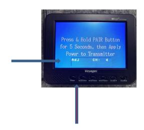
3. POWER ON MONITOR AND SELECT THE CAMERA INPUT USING THE SELECT/PAIR BUTTON ON THE MONITOR
