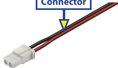
Canbus Terminating Resistor
