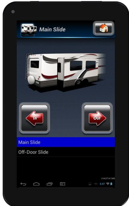
III. Pressing "Out" will extend the slide-out (Fig. 32A).
