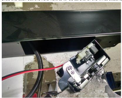
5. Remove the wires from the actuator and then undo the nuts and bolts that hold the actuator into the latch assembly.
