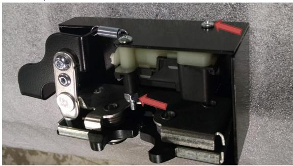
6. Install new actuator. When re-installing the latch assembly the wiring needs to be hooked up the correct way. The actuator has a raised area on one side, with that down, the red wired goes to the left. It is always best to connect the wires and then cycle the key to make sure you have it hooked up correctly.
