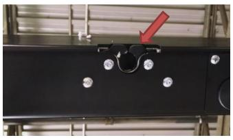
3. Remove the 4 button head cap screws holding the latch using a 5/32" allen wrench
