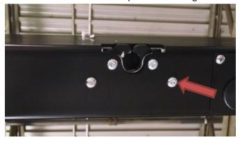
4. Slide the latch out the hole next to it. Be careful of the wires attached to the actuator.
