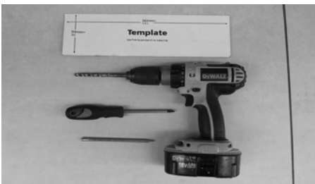
15 Tools required ● Pencil or fine point marker ● 1/2" to 1" drill bit ● Jigsaw or sawzall ● Cut out template (included) ● Philips head screwdriver No 2
