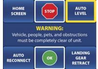
The system will go through a series of moving the jacks and checking the unit for level. The display will read "AUTO LEVEL IN PROGRESS". When the system has successfully leveled the unit, the display will read "AUTO LEVEL SUCCESSFUL" and a beep will sound.
