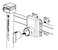
Fasten with the included Stow/Clevis pin. Then, set the cotter pin through the Stow/ Clevis pin. These pins are to be removed when either detaching or stowing the jack.
