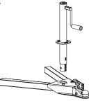
You can now fit the jack to the coupler. Bolt sizes are specific to your coupler and are not included with your JX purchase. Alternatively, the center jack can also be welded for a more permanent attachment to the trailer.
