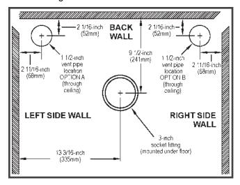
Position the tank against three walls. Mark four holes at mounts on tank base. After holes are marked, remove tank, and drill pilot holes. Slide tank back into position. Secure the tank with four screws and washers on all tank mounts.
