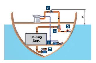
1 Seawater pump 2 Stop cock 3 Vent 4 3 way valve 5 Discharge of the toilet direct to the sea 6 Gravity drainage to the sea of the holding tank 7 Discharge to the sea of the holding tank
