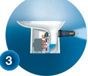
Waste is then discharged through a standard 1" or 1-1/2" pipe.
