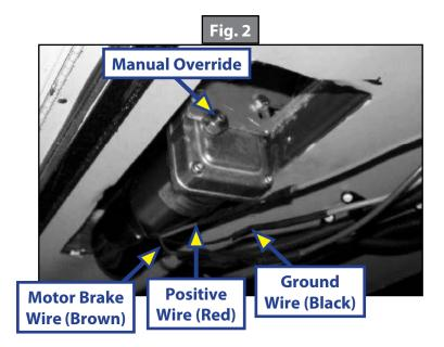
2. With a second person assisting, one person must push and hold the manual override switch while the other person, using a <sup>5</sup>/<sub>8</sub>" wrench or socket/ratchet combination, rotates the hex head manual override (Figs. 3 and 4) to manually move the slide-out.
