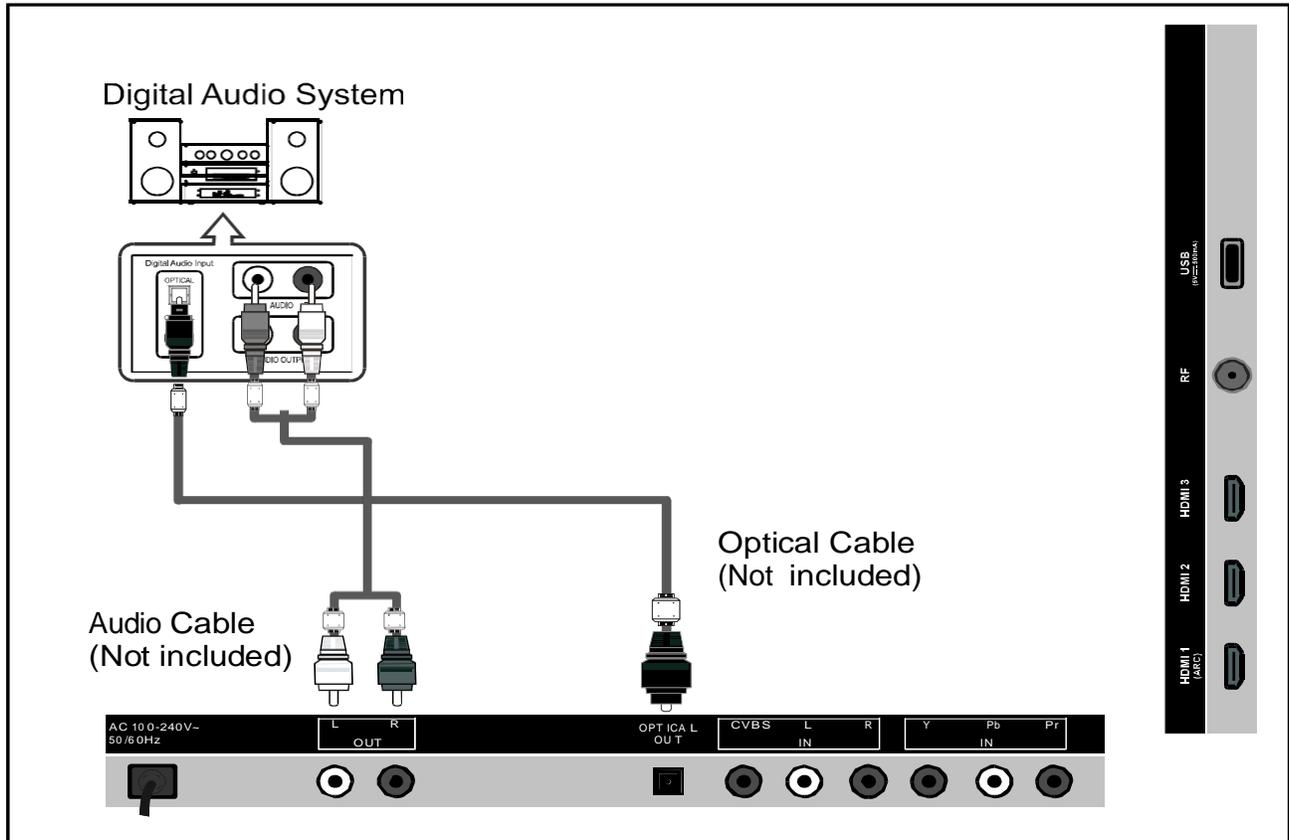
5.1 CH audio is possible when the TV is connected to an external device supporting 5.1 CH. We recommend the use of cables with a Ferrite Core.
