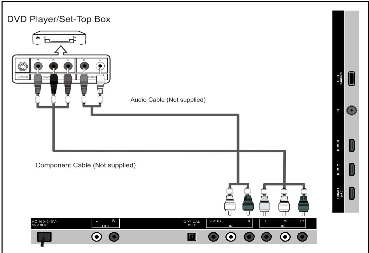
Component video separates the video into Y (Luminance (brightness)), Pb (Blue), and Pr (Red) for enhanced video quality.
