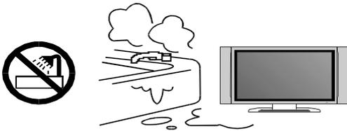
The LED TV should be kept free from rain, moisture and dust to prevent electrical shock and short circuits. Do not cover the ventilation openings with table clothes, curtains, newspapers, etc.
