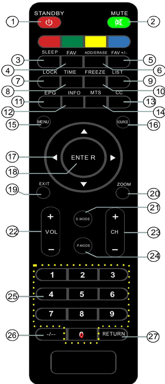
1. STANDBY: Switch LED TV when in standby mode or vice versa.
