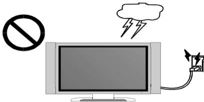
Pull out the power cord and antenna cable during electrical storms so the LED TV is not damaged by electrical surges. Keep all people away from the antenna cable during electrical storms.
