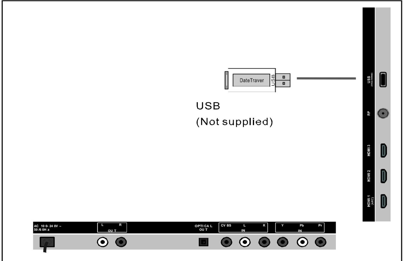
Connect a USB 2.0 memory device into the USB slot of your TV for playback of multimedia files.
