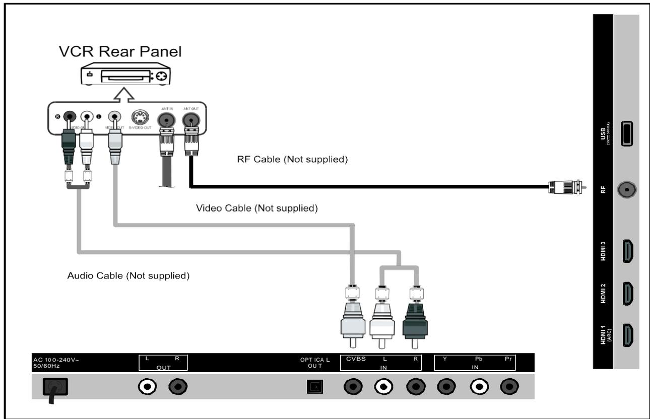
Follow the instructions in Viewing a VCR or Camcorder Tape to view your VCR tape. Each VCR has a different back panel configuration.
