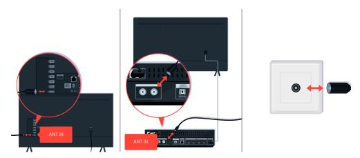
Check the antenna and input cable connections.
