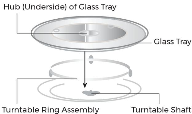
(1) Place the turntable ring in the round depression in the bottom of the microwave oven so that it turns freely.
