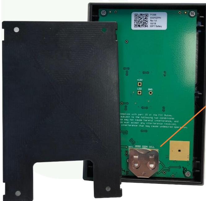
Slide the battery up to remove.
