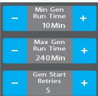
Minimum Gen Run Time - Use the +/- buttons to set the minimum amount of time that your generator will run once it has started. (Range 10min – 30min)
