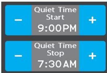
Quiet Time Start - Use the +/- buttons to select the starting point for Quiet Time, the hours that your generator will not run in an effort to reduce noise.
