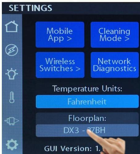
Tap to select the required Model, Floorplan and Options for your specific vehicle. Tap Apply to save and exit.
