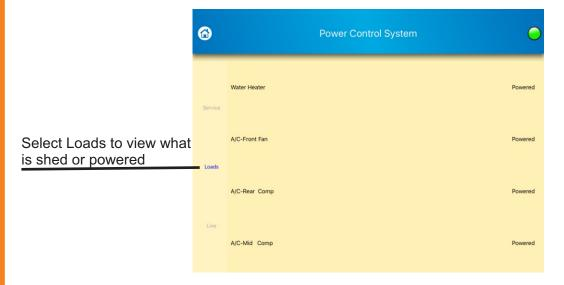
This image shows that all the air conditioners and the water heater are powered. If someone in the RV starts using a lot of power (running the microwave, hair dryer, etc.) the water heater and air conditioners would shed their power to prevent a trip in the order they're listed. They will take two minutes to restore power after power becomes available again.
