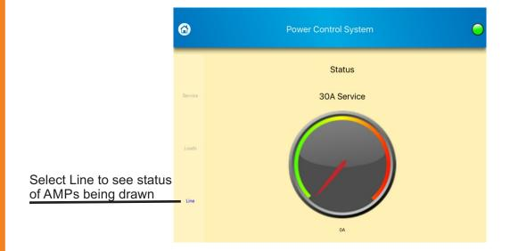
By selecting Line, the user can view how many amps are currently being drawn by the entire RV. When amps being drawn by the RV exceed the service available, the PCS will automatically start shedding loads to prevent circuit breaker tripping.
