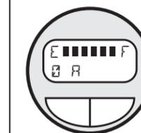
The SoC LCD Display (PN: 881-0401-12) on the system remote panel powers up whenever BMS is turned on. Its screen has two lines where battery information is displayed.
