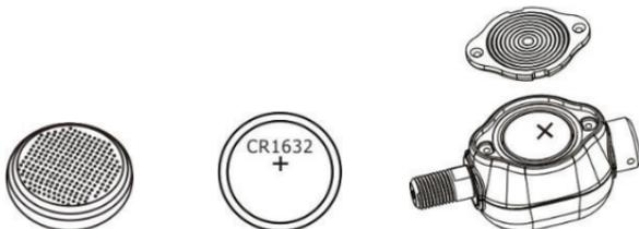
**NOTE:** It is recommended that you check the voltage of the new battery before installation. It should read 3+ volts when new. Do not install if the battery reads less than 3 volts.
