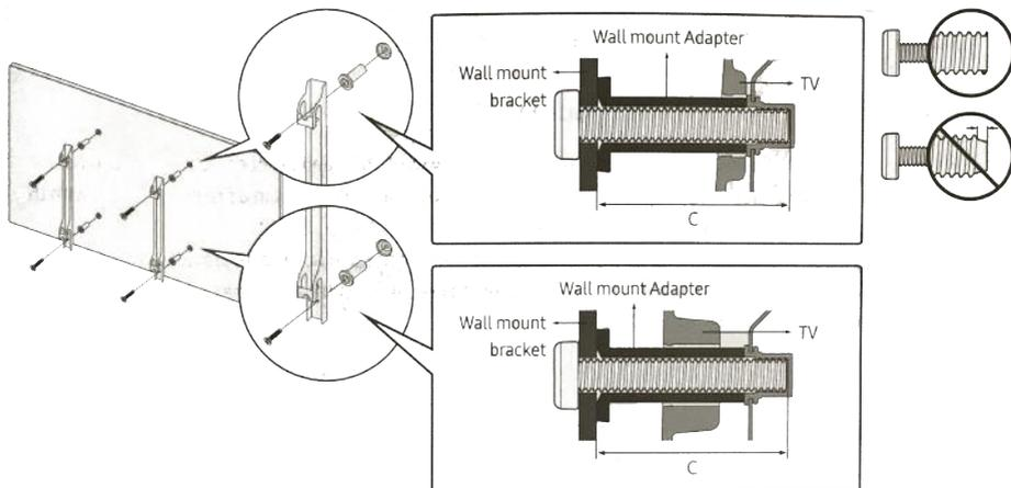
1. Assemble the wall mount adapter.
