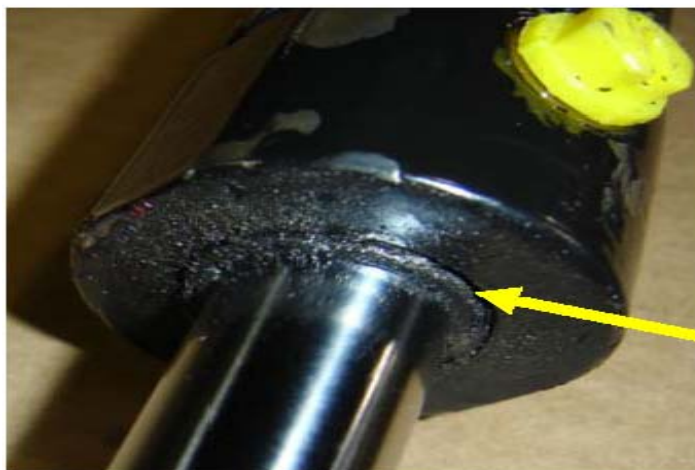
Paint Residue Collected at gland seal.
