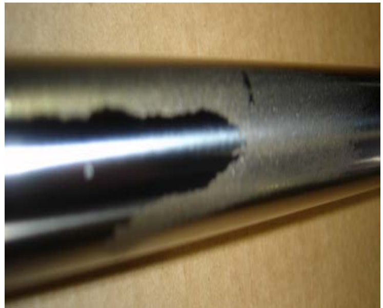
Paint On: Cylinder (Ram) Shaft
